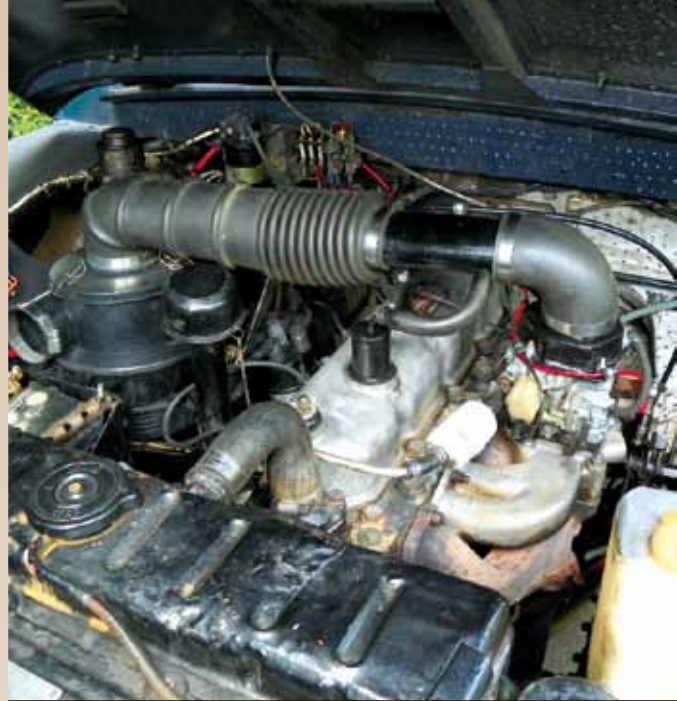
2.286-litre 4-cylinder first fitted to Land Rovers in 1958.
