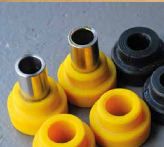
A set of modified polyurethane bushes will replace the Vesconite ones originally made to locate our radius arms. It's amazing what can be achieved quickly by people with the right skills and equipment so it's a big 'thank-you' to RGMotorsport for not beating about the bush.
