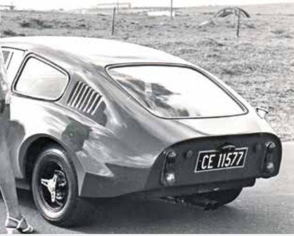
According to Kamm's theory a truncated teardrop shape is more aerodynamically-efficient when its tapered point is replaced by an abrupt chopped rear end.
