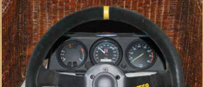
It's called the knock-on effect and it complicates custom car builds: the E36 gearbox doesn't have a speedometer drive, so we changed to this Stack unit, with a pick-up at a front wheel.
