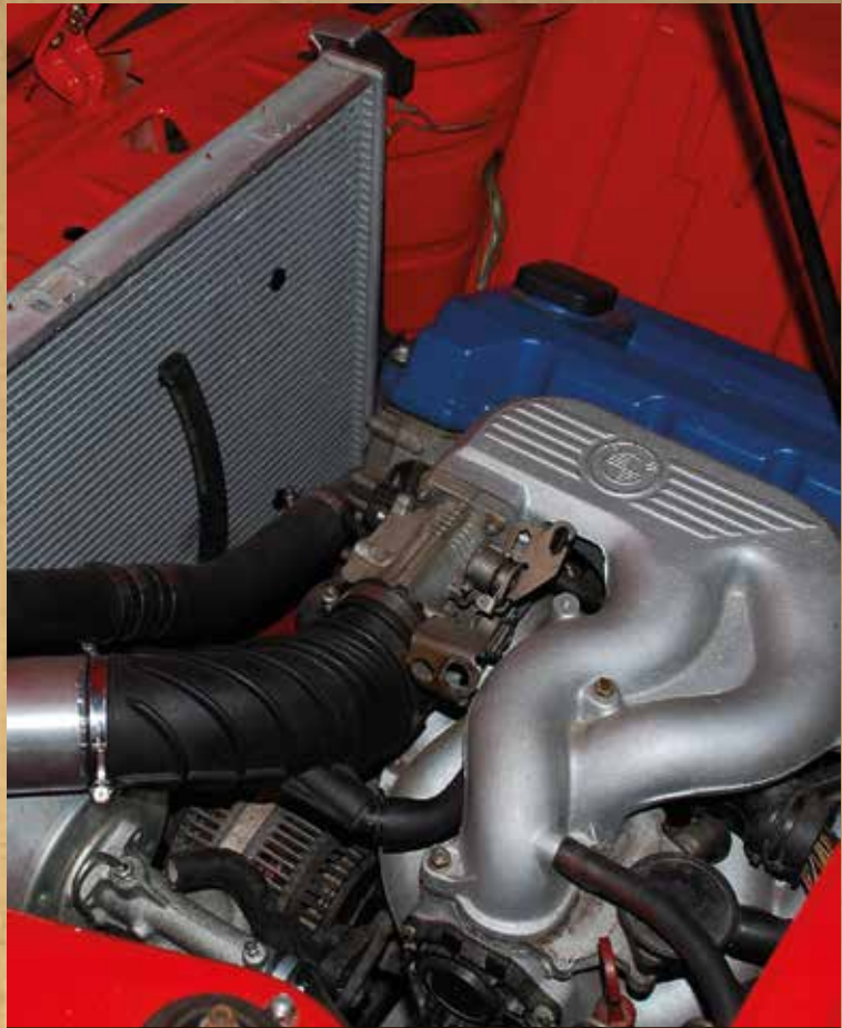
M44 engine didn't fit like a glove... RGM built the custom air intake, Norbrake did the hydraulics (making use of a single booster). Where's the battery? In the boot, where it's found on most performance Beemers.
