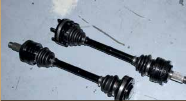
Sajco made up these custom driveshafts to combine a 2002 differential with 325i hubs and brakes.
