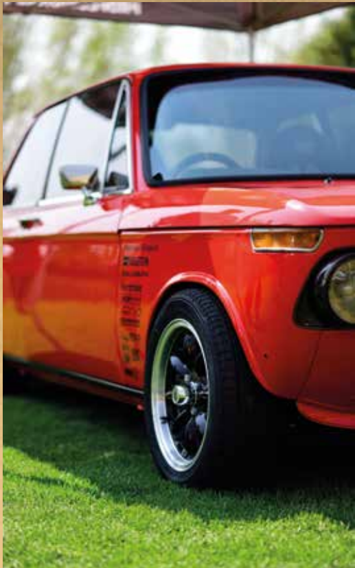
Paintwork plus black chrome bumper treatment makes for a nice contrast. We've gone for a stagger on the tyres: the rear Dunlop SP Sport LM704s measure 205/50/15 and at the other end 185/55/50. It's a high performance tyre, providing good handling and excellent wet grip – just what a 2002 needs! Byline Chris Wall Media
