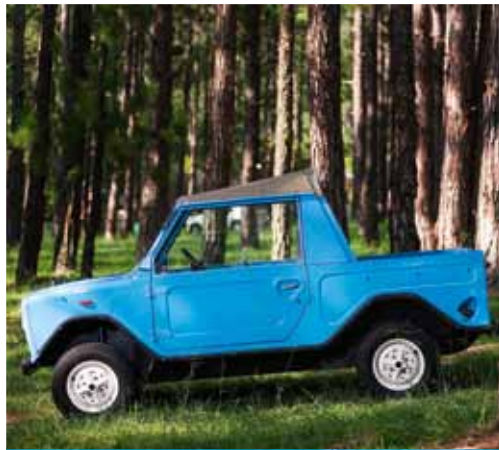
Small front and rear overhang helps approach and departure angles.
