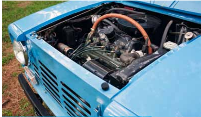
Famed A-Series engine mounted transversely.
