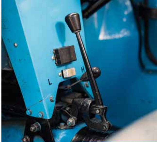
Basic center consul showing lever for high and low ratios.
