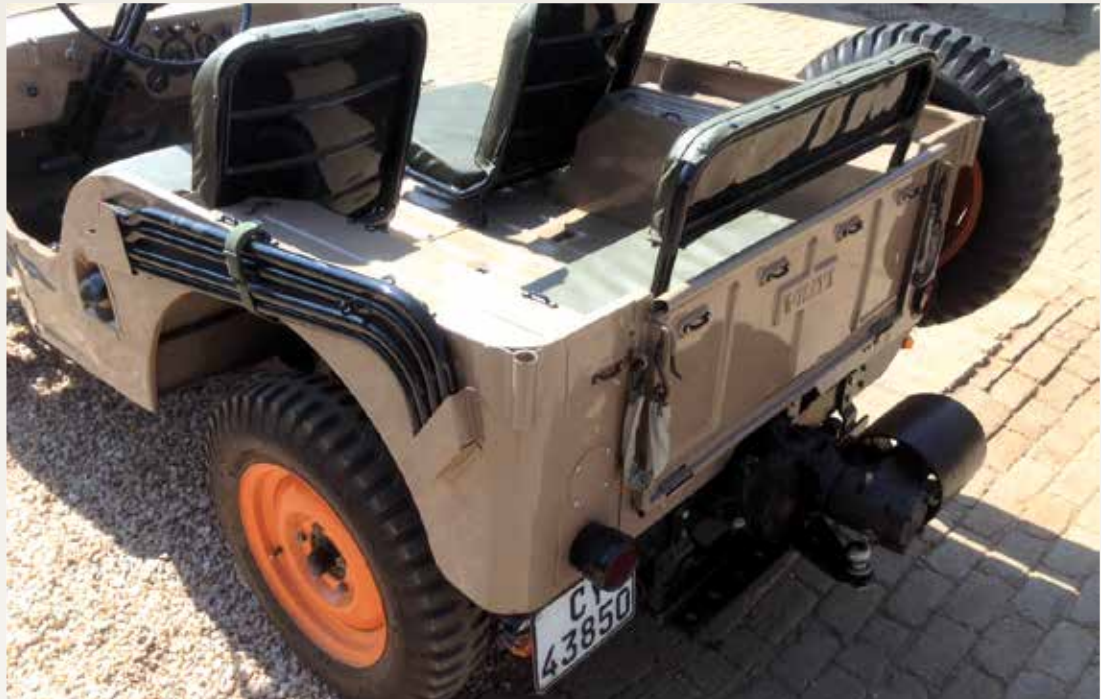
Removable tailgate, the canopy frames neatly stored in brackets and the heart of the matter, the PTO to drive implements. Image: Claus Heydenrich.
