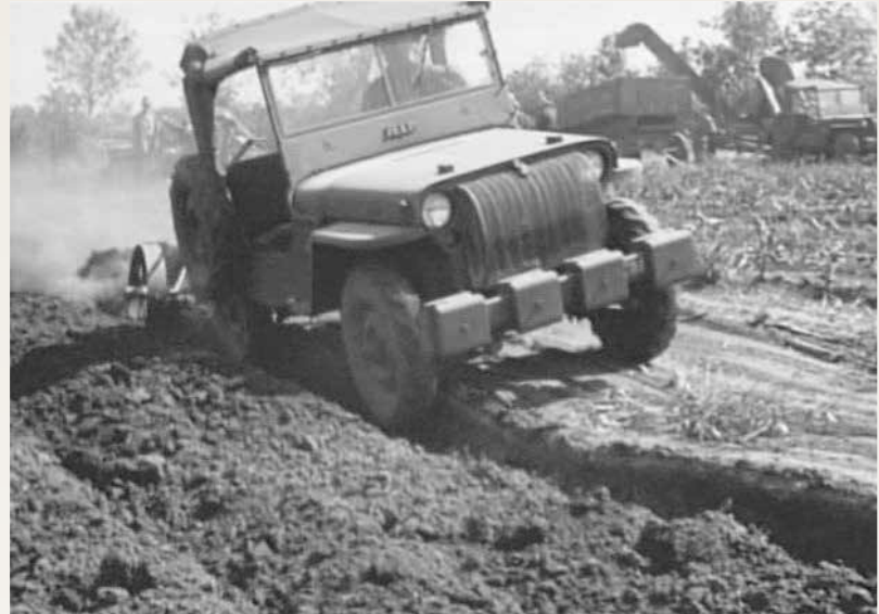
A CJ2 ploughing. Notice the bumper weights to keep traction on the front wheels.
