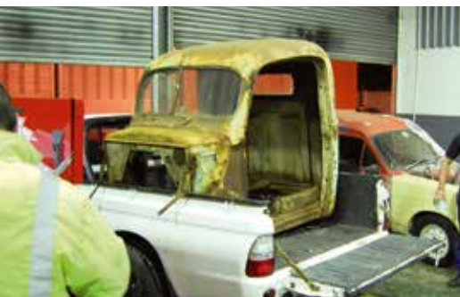
Going to get new floor and firewall.
