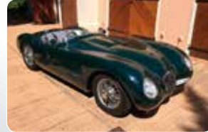
1951 Jaguar C Type Replica, British Racing Green with Green leather seats, built by Nostalgia Cars UK, Fibreglass body, space frame chassis with Aluminium panels, 4.2L XJ6 Motor, 5 speed manual gearbox, disc brakes. POA
