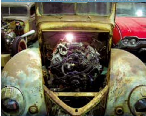
Cab in place, mocking up front sheetmetal.
