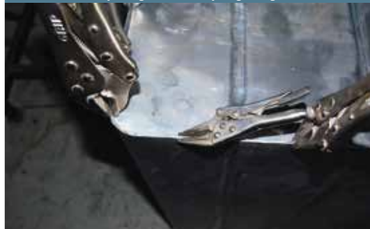
Ready to weld the seam.
