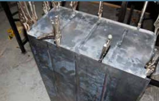
A new 95litre fuel tank was made.
