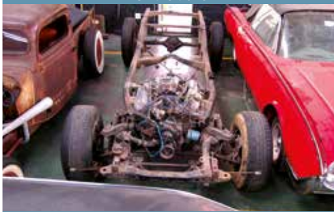
Courier rolling chassis with engine moved back.
