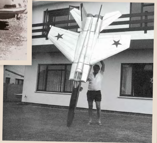
John's 1/3-scale model MIG jet powered by two 10cc two-stroke engines driving propellers.
