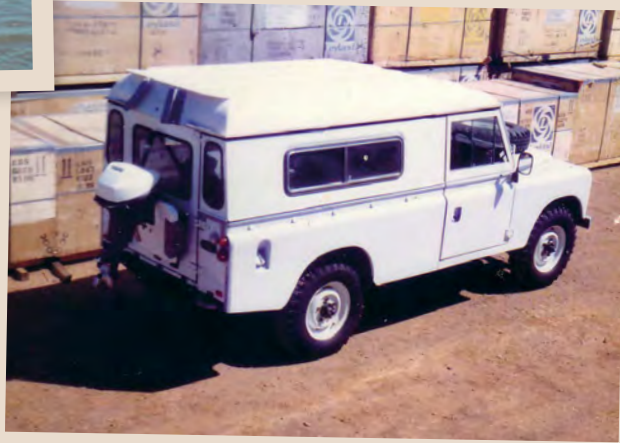
The Land Rover boat was designed to be carried (inverted) as the roof panel of a 109in Land Rover with the engine hooked on to the back door.
