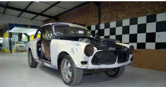
Despite being good solid cars this Volvo suffered rot in the floorpans. New pans were fabricated and fitted. Next job is to prepare for paint.
