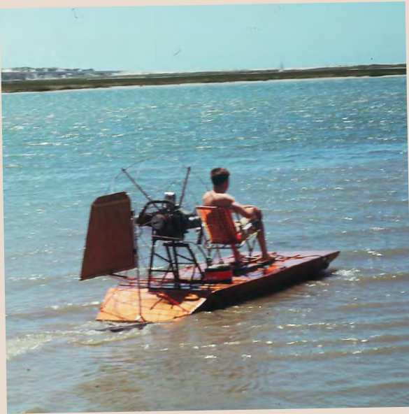
His self-designed and built swamp boat was powered by a two-cylinder Goggomobil engine.
