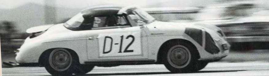
Racing at St Albans. The engine lid was raised to promote downforce.
