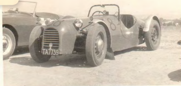
"Mulgaf" special - Brian Newby - based on Fiat front and rear suspension 1954/5
