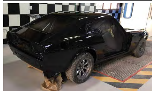
This 260Z came in bright yellow but the client wanted it black. Black exaggerates any bodywork flaw so it was imperative to get every panel spot on before shooting the paint. We think the owner made a good call on the new colour.
