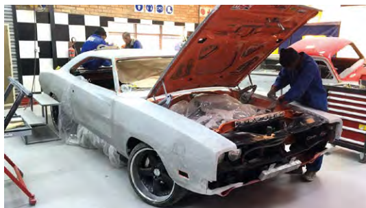
Although supposedly fully restored when purchased recently, an inspection revealed numerous filler covered rust spots on this Charger. The remedy was to cut these out and replace with metal. Final panel beating being done before full respray.
