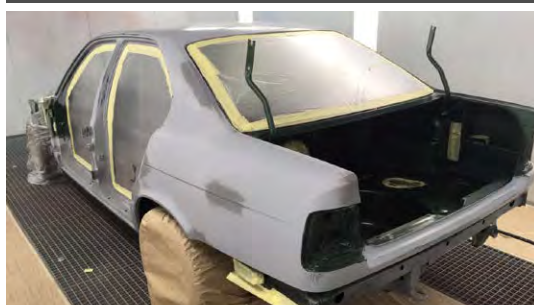
With rotten inner and outer sills on both sides of this rare Alpina BMW the only option was to fully remove the sills, find some structurally sound ones from a donor car and weld them in place. Job done the car now gets a new lick of paint.
