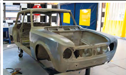
This Alfa Romeo Giulia is nearing the point where a deep blue colour can be applied. To get to this stage metalwork has been done to remove any rust and all the panels fitted to ensure accurate gaps.
