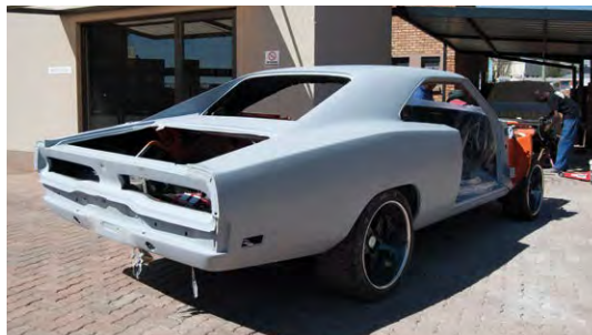
Poor previous restoration work has meant that this Charger has had a full redo. Metal has been cut out and replaced and the engine removed to repaint the engine bay. Ready for paint, it will be with the owner soon.
