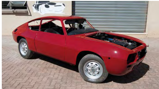
The Lancia Fulvia Zagato is now ready for trim and assembly. Rotten metal was replaced and the correct colour applied – made possible thanks to the car having the original paint tag in place and it tying up with Glasurit's paint library.
