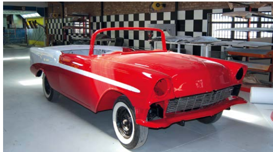
This 1956 Chevrolet Bel Air has arrived blue and has been stripped all the way down and resprayed in a brilliant red and white scheme. It is ready for assembly.
