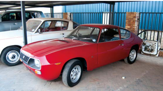
A very rare Lancia Fulvia Zagato is now ready to be collected by the owner. The car was completely stripped and rust replaced with metal before the original colour was applied and trim fitted.
