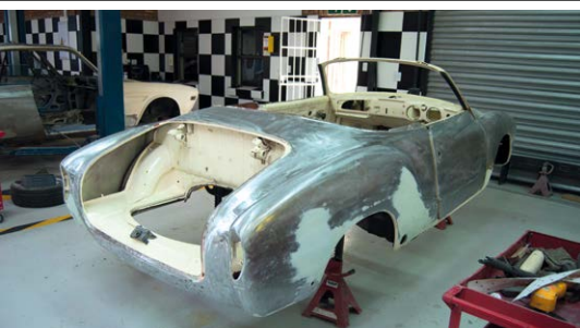
New arrival Karmann Ghia cabriolet. It has been down to the metal and is in surprisingly good condition. A few details will be sorted before primer and paint is shot.
