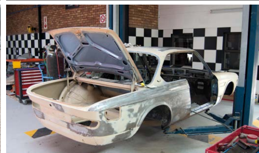
The BMW CS we started last month is making progress. Although the body is good the floorpans were rusted through – These have now been cut out and replaced with new metal.
