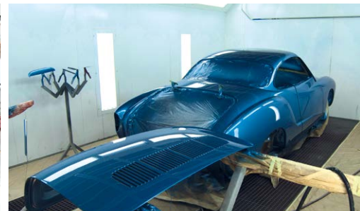
A customer stripped this Karmann Ghia, which helped speed up the time frame but there was still hours spent on prepping the body for this brilliant blue hue. It is ready for the client to assemble.
