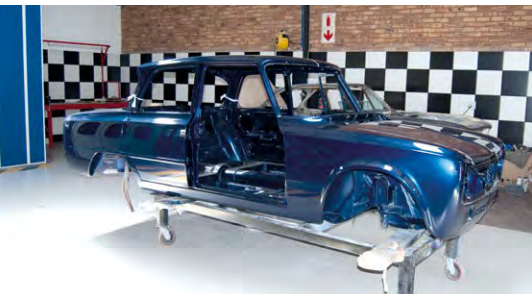
This Alfa Romeo Giulia arrived as a bare shell. Dents, rust and body preparation was done before shooting in a deep blue borrowed from the Maserati colour chart. The client will assemble.
