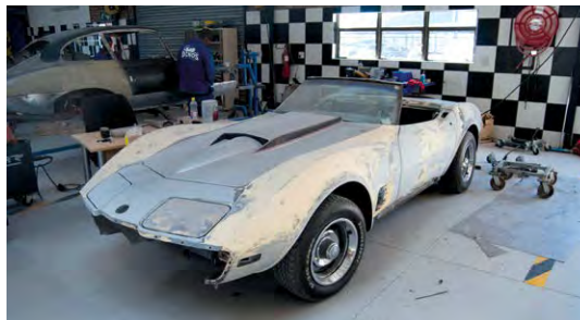
Having stripped down this Chevrolet Corvette the body has been prepped and is awaiting parts to enable proper bonnet fitment before being primed, painted and assembled by Dino's.
