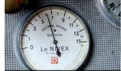
Nivex vacuum petrol gauge is fully functional.
