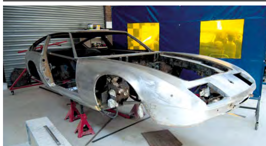
Arguably the largest job on the go at the moment this rare RHD Maserati suffered in the rust department heavily. To date new sills have been made and fitted and hand-formed floorpans have been added. This meant real old school skills, even down to making the correct tools to do the job.
