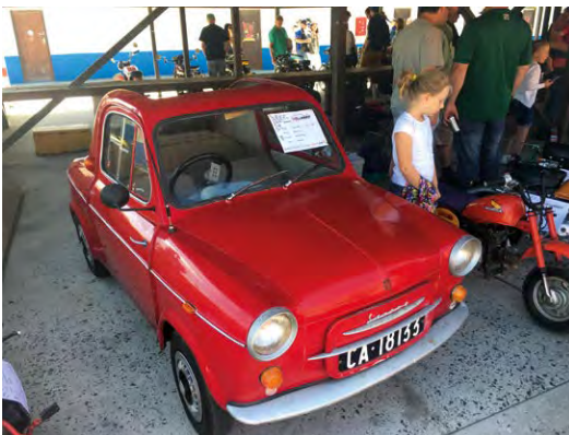
The extensive motorcycle displays included this 1960 Micro car , designed by Vespa but built in France to avoid compromising Fiat 500s sales in Italy. It features a 14bhp 393cc twin-cylinder air-cooled engine.
