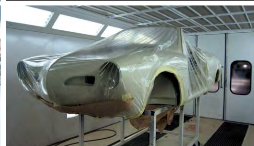
The client dropped this Karmann Ghia body off for rust and dent removal before the shell was prepped and painted. With the body done the inner wheel arches are being protected against stone damage and the client will collect to assemble.
