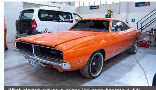
What started out as a minor job soon became a full body job when rust covered over by the previous builder was uncovered. This has been remedied, brilliant new orange paint and graphics applied and is undergoing final assembly.
