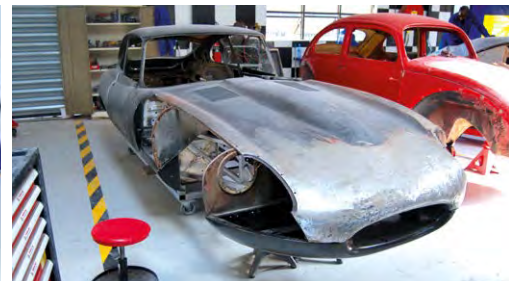
Another job we took down to the metal in order to cut out rust. The E-Type is now being fitted with brand new imported reproduction parts. Despite being made for this vehicle the replacement parts never fit 100% so a lot of fine tuning and panel fitting is being done.
