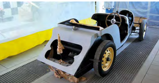
This very rare 1936 Morgan is the oldest machine in the shop at the moment but arrived in a surprisingly solid form. A few dent and metal repairs have been carried out and the body is ready for paint. Research into what the original colour was is underway.
