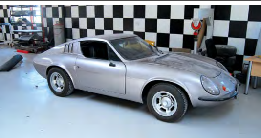
Only ever built in Brazil and South Africa the Volkswagen based Puma GT is fast gaining traction as a collectable classic. Fibreglass technology wasn't to the standard it is today and years of flexing and DIY paint mean that this one needs a full respray. The vital surface preparation will start soon.
