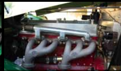
1271cc K-Type Magnette engine.
