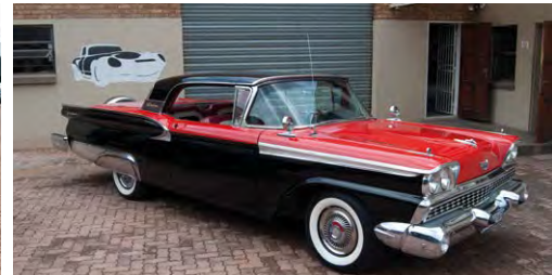
Despite only repairing this Ford Galaxie's doors, sill and front wings we feel like we have worked on an entire vehicle – it is the biggest car to have come through the workshop. Panel gaps were not good when this behemoth arrived but hours of adjustment have them spot on and make the world of difference.
