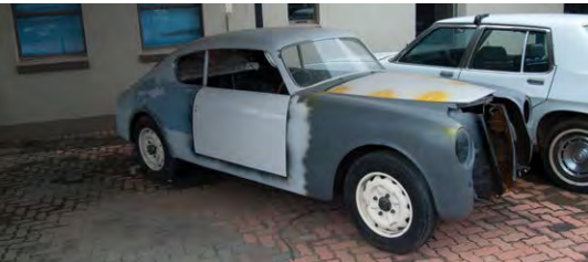
This rare Lancia Aurelia has just been delivered by an overseas client for full restoration. As can be seen a previous owner/panel beater stripped the vehicle years back but never got around to finishing the job. We will start from square one. Loosely assembling the body to assess the work required and then take it back to a bare shell to start the hard graft.
