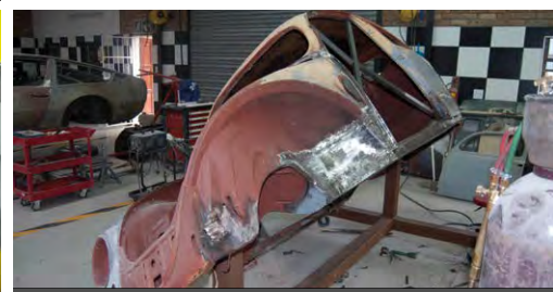
This split window Beetle has suffered the ravages of time. Not only did it have numerous dents and rust areas but it also suffered some poor repairs previously. They are a rare find now so worth going the whole hog back to bare metal before cutting and replacing where required. Here braces hold the body in shape while the undesirables are cut out and replaced with shiny new metal.
