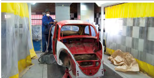
Repairs have been done to this Volkswagen Beetle body and it is now being readied for primer and paint. The owner will complete the assembly and restoration himself. By the time he takes delivery it will be as good as, if not better, than a body the factory body shop supplied to the production line.
