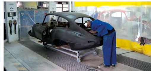
Following a bare metal exercise where a large amount of rust was removed and new metal put in this Jaguar E-Type is nearing the point where primer can be applied and then paint. The initial black primer visible was put onto the exposed metal to stop hand marks leading to any corrosion while still being panel beaten. Black is also good at showing up any imperfections before painting.
