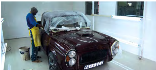
This Ford Prefect has been a carryover from last year with a large amount of metal work taking place. It was converted to a bakkie (by using a Cortina loadbin) with large wheel arch flares years ago but the quality wasn't that good. It meant Dino's had to cut out large portions of rust and remove loads of putty and fibreglass. New metal has been added, paint applied and is now seeing final trim fitment and finishing.
