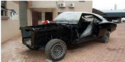
A 440 Dodge Charger undergoing a colour change. It has been stripped to the metal and minor dent and rust repair carried out. The first paint coat, including full engine bay, has been applied. Panel assembly will now take place and a second coat of paint put on. For depth a double clear layer coat will then go on.
