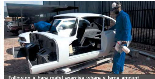
Following a bare metal exercise where a large amount of rust was removed, new metal put in and panels fitted, this Jaguar E-Type has finally reached the primer stage. Hours of work went into getting the specially-ordered reproduction nose to fit – it is worth remembering that even though you can buy replacement panels, they will never fit exactly and need plenty of fine tuning.
