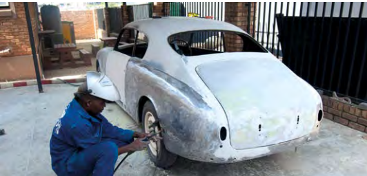
On arrival this Lancia Aurelia was partly assembled and looked in reasonable condition. We loosely assembled the car to see where we stood. From there the multiple layers of paint were stripped off, sadly revealing a host of poor repairs neatly covered by thick filler. It's all off now and lots of welding and metal shaping hours lie ahead.
