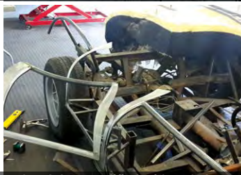
A donor 400i chassis and running gear was sourced and then modified with a skeleton to support the new aluminium bodywork.
