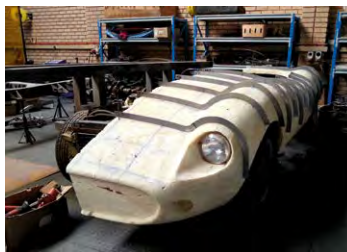
Having aborted the wooden buck polyurethane foam was laid over the 400i chassis and then hand carved as a former for the final shape.
