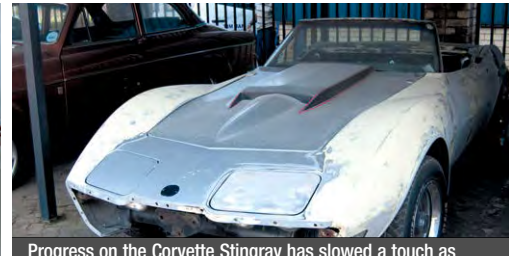
Progress on the Corvette Stingray has slowed a touch as we wait for some bonnet fasteners from America. The chances are the fitment of these will mean realignment of panels is necessary. This will require lots of hands on the bodywork so it's best to do the surface preparation after that. Thereafter the paint can be done – in this case as per the original.
