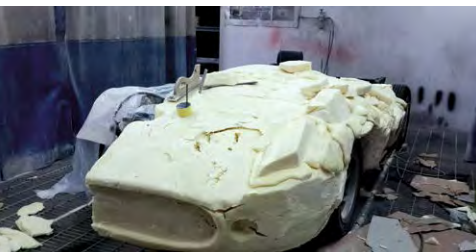
Having aborted the wooden buck polyurethane foam was laid over the 400i chassis and then hand carved as a former for the final shape.
