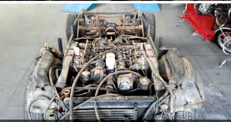
A donor 400i chassis and running gear was sourced and then modified with a skeleton to support the new aluminium bodywork.
