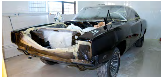
This 440 Dodge Charger was in reasonable condition when it came in but the owner wanted a colour change. It has been stripped to the metal and minor dent and rust repair carried out before a first coat of paint was applied. Panels were then fitted and a second coat of paint has just been completed. With a double layer of clear coat the depth of the paint is brilliant.
