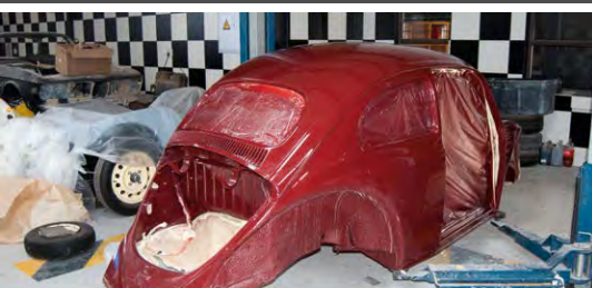
Repairs have been done to this Volkswagen Beetle body, the primer and preparation stages went well and the result is a show-condition final paint job. Masking will now be removed and a polish done before handing over to the owner who will complete the assembly and restoration himself.
