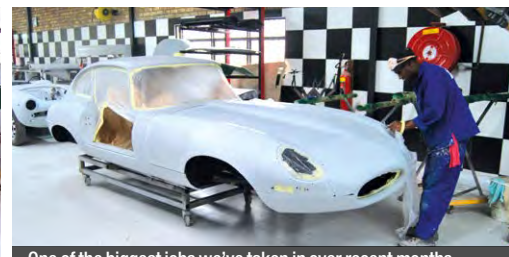
One of the biggest jobs we've taken in over recent months, this down-to-bare-metal Jaguar E-Type had hours of rust cutting and new panel fabrication. Even fitting the imported new bonnet took plenty of tweaking to get the fit just right. It heads into the spray booth this week and will come out looking as good, if not better than, new. The owner will assemble the car.
