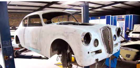
Except for the incorrect nose this 1953 Lancia Aurelia looked in reasonable condition on arrival but with the paint stripped, numerous previous poor repairs were revealed. These have been cut out and new metal added, and a new front nose made to suit. It's ready for primer and paint now
