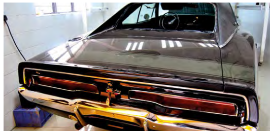
This 440 Dodge Charger is nearing completion, with the last few bits of trim and brightwork being added on. Regular readers will recall that this car came in for a full colour change so was stripped down to metal and all the minor imperfections repaired, before shooting the car in black with a subtle green bumble-bee stripe.
