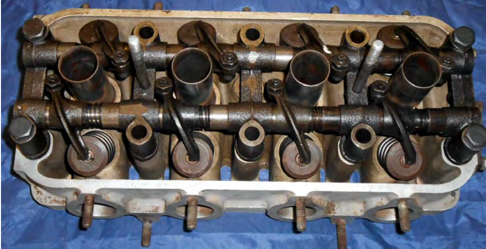
Crossflow cylinder head with twin overhead rocker shafts driven by the single block-mounted camshaft.
