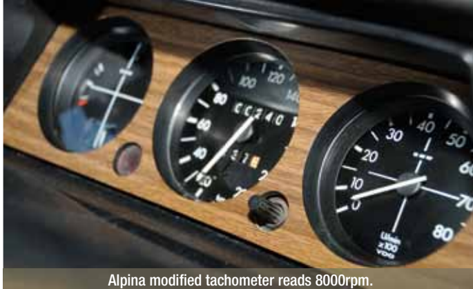
Alpina modified tachometer reads 8000rpm.
