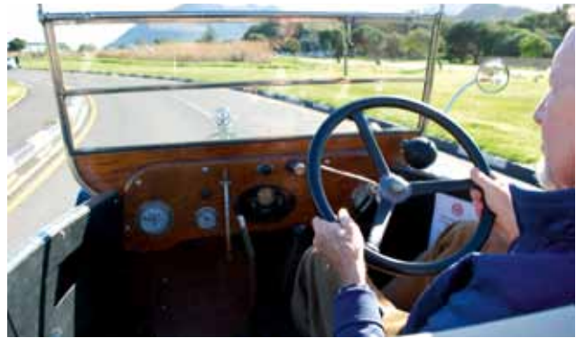
Accelerator pedal is in the middle and the use of foot and hand lever brake is required.
