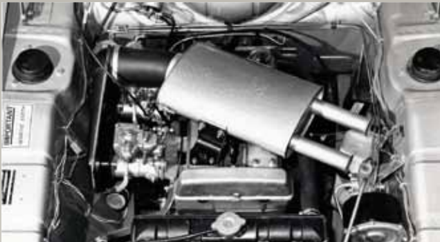
1.6-litre DOHC was good for 82kW and 145Nm of torque.
