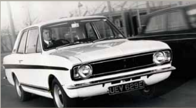
The only cosmetic difference between an entry level Mk2 and a Lotus were the 5.5 inch wide wheels and black grill.
