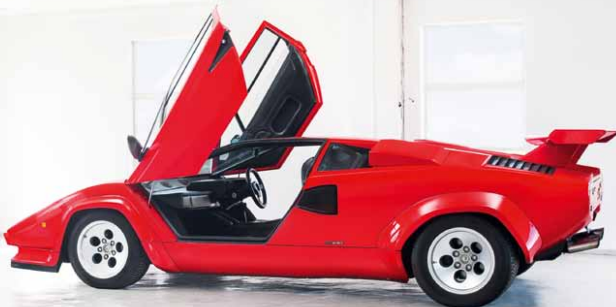
Hardly a curved panel on the aircraft-grade aluminium body over a tubular chassis. Scissor doors became a Lamborghini symbol.
