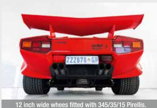
Hardly a curved panel on the aircraft-grade aluminium body over a tubular chassis. Scissor doors became a Lamborghini symbol.
