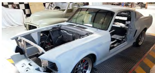
Ready for paint. This Eleanor Mustang recreation was in good shape when it arrived but the owner wanted it even better. Panels now fit brilliantly and the surface has been taken back and prepared for a deep paint finish as per the movie Gone in Sixty Seconds . Dino's will reassemble.
