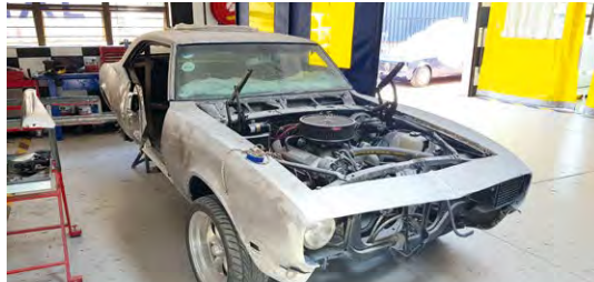
Readers will have seen this Camaro last month. It drove into the shop but when stripped revealed a lot of hidden rust. Hours have gone into cutting out the bad bits in the sills and rear wings and it is approaching the point where primer can be applied.
