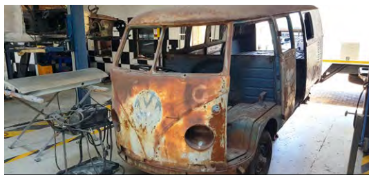
This Kombi takes it to the Charger in terms of biggest project of the year so far. It has lived a hard life and every panel has severe rot and damage. We've cut out portions of the side and replaced with new metal and will get cracking on making up new nose pieces rather than importing reproduction items.
