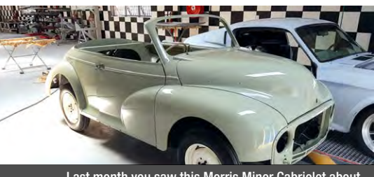
Last month you saw this Morris Minor Cabriolet about to enter the spray booth. Today you see it in all its fresh paint glory and awaiting the owner, who will put it back together. Being such a rare model it is pleasing to see that the original colour was selected from the Glasurit library.
