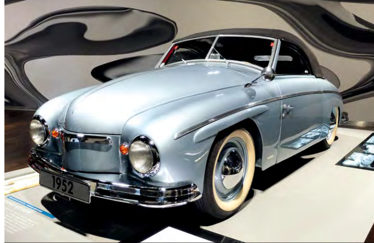
Johannes Beeskow designed the pontoon-shaped bodywork of the Rometsch, which is based on a Beetle platform. This attracted many celebrities to the brand.
