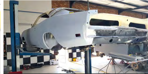
Our biggest project so far this year. This Dodge Charger suffered badly in the rust department and we've had to replace everything (including chassis rails) but the roof, bonnet and doors. Most replacement parts are available but the odd one has been handmade.
