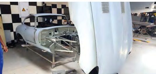
The end is in sight for this long-term E-Type project. The imported nose section has taken an incredibly long time to get fitted correctly and we had to cut a lot of corrosion out of the original body. The interior has been painted and it is ready for its outer coat.
