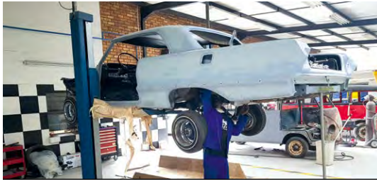
This Impala has had the paint removed and numerous sections of metal replaced on the outer body. It is now on the lift to get to the underside where a few gremlins lurk in places like the boot area. A sturdy floor is needed to house the control system for the trick adjustable hydraulic suspension in this low rider.
