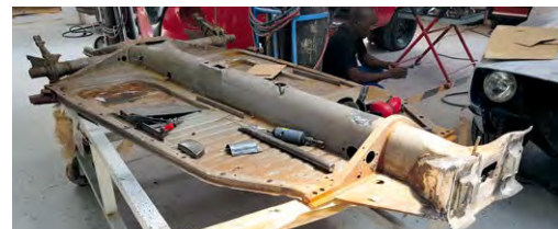
The owner of many of the air-cooled projects we've done recently has brought this Beetle pan in for repair. While it is possible to buy a completely new pan, he feels that this might lose some of the heart and soul. It will take time to straighten and replace the metal, and will probably cost a similar amount to buying a new part, but it will keep the originality.
