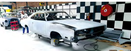
We said the rusty Kombi might be the largest job of the year. It is not. This Dodge Charger is ready for paint. To get it this far we've cut away most of the car. We've imported or made up a new floor, door, firewall, chassis rails, wings... and the list goes on. Once painted, the owner will ship it off to install a hulking V8 and new running gear.
