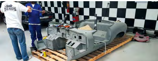
With the E-Type coupé ready for collection, the owner has dropped another E-Type project for us to do metal work and paint on. It was imported from the States and we can immediately see holes in the floor and sill areas. These will be cut out and new metal applied. The owner will source new replacement panels should the need arise.
