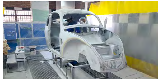
It took a fair amount of fabrication to fix rotten panels in this oval window. The rear valence, for example, was made up from scratch. But the end is in sight with final preparation for paint being carried out. Once painted, the client will take the body away and complete the build.
