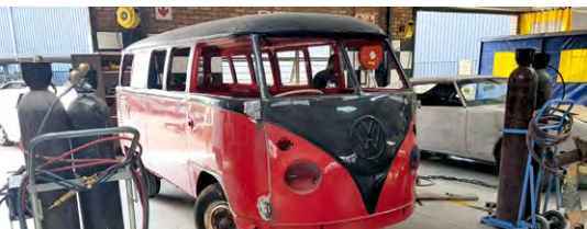
These split-window Kombis are all the rage and finding a good one is getting difficult. This one, although sporting rust in most parts, is relatively good. We are lining up all the panels before stripping and bracing the shell for any metal removal that needs doing. Once the body is done, the owner will collect and finish.
