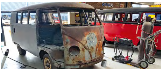
See what we mean about the red splittie being relatively good? This one is far from it and is up there as the biggest job of the year so far. We've cut loads of tin worm out the side and thrown some primer on to preserve that while we get cutting and making new floor sections. Then we'll tackle the nose job. Only then will the paint prep start.
