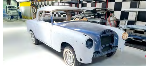
As mentioned before, this Mercedes-Benz 220S 2-door had a recent paint job. Wary of applying new paint on top of this, we've stripped the sides and uncovered some issues that have now been remedied. Next we will do nose and roof and then paint in the two-tone scheme before the owner takes it home to put it back together.
