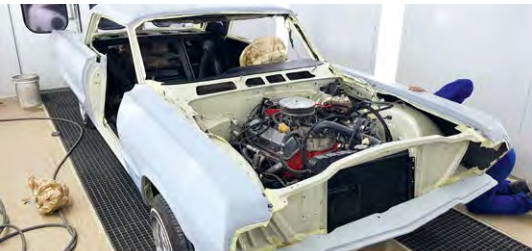
The low-rider Impala is in the paint booth. We've shot the engine bay and now will lay on the exterior hue. Of course, to get it to this level we took the body down to the basics and had to fix a number of issues. It is going to be a showstopper.
