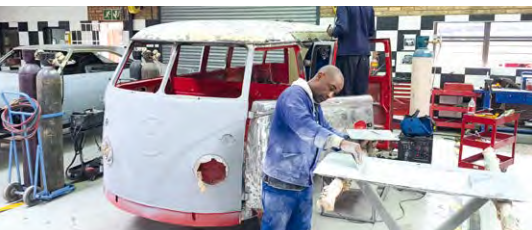
These split-window Kombis are all the rage and finding a good one is getting difficult. This one looked good on the surface but stripping revealed plenty of rust covered by fibreglass. We are busy making new roof sections and will then get stuck into the other poor areas.
