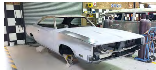
We said the rusty Kombi might be the largest job of the year. It was not. This Dodge Charger was. It has new floors, doors, firewall, chassis rails, wings... and more. It has been on hold while the owner decided what powertrain he wanted. But having decided on original it will go in for paint soon.
