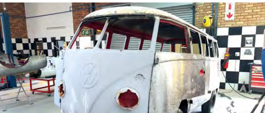
This split-window kombi didn't look that bad at first glance but once the stripping was started it revealed its dark side – fibreglass patches over rusted areas were prolific. We've made a new roof section and added plenty of new metal to the front section. Now we are on the cheese-like holey floors. It goes to show that when it comes to buying resto projects, the honest unpainted old 'skadonks' are often better options than something with a fresh lick.
