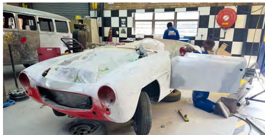
Another car that looked ok with some recent paintwork, this SL190 had more to it than met the eye. When stripped back to the metal it showed hundred of small dents (possibly caused by hail) that had simply been filled with Bondo and then painted. We've spent hours panel-beating these out and are now making sure the panel fit is spot-on before primer and paint.
