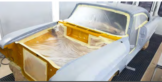
This Dodge was a solid, original car but we took it down to the basics to repair any niggles and also allow for a full colour change. The owner has chosen to move from the light metallic brown to a bright yellow. The engine bay and hidden areas are done and now the exterior happens. Dino's will assemble the car fully when done.
