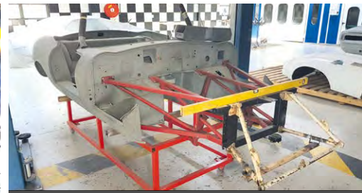
The E-Type Jaguar – arguably the most beautiful car ever made. But this one, the second for the same client, has a long way to go to meet this status. The floors are almost non-existent and the rust has had a serious go at the sills, rear light surrounds and even bonnet. We are mocking it up before starting the surgery to ensure things are straight.
