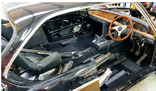
Our very own BMW 3.0CSi is progressing reasonably well. The body was stripped, repairs carried out and a deep black colour shot. Assembly is underway and we're making strides on the interior. The seats, dash, carpet and wood veneer have all been done in SA and are exceptionally good.
