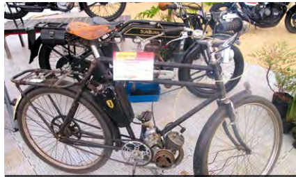
This was one of the original 'help my trap' mopeds, a 1956 Zundapp 50cc engine fitted to a bicycle.
