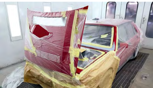
One of rallying's most iconic cars, this Lancia Delta Integrale has come in for some minor rust repairs, touch-ups and general TLC. We've cut out the damaged areas and replaced with new metal. The surfaces are being prepared before paint is blended in to match seamlessly.
