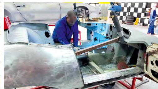
This Jaguar E-Type is a big job and is taking time to get just right. The floors, sills and boot were almost non-existent, with the tin-worm having been busy. Replacement sections have been imported but even though brand new, they will never fit 100% so we need to spend hours tweaking them.
