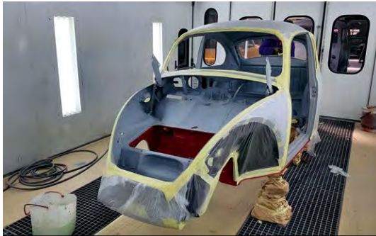
Another Beetle nearing completion and delivery to the client for assembly. The regular amount of corrosion was removed and replaced with hand-shaped new parts. With the underside painted in the correct red, it’s time to shoot the upper body.
