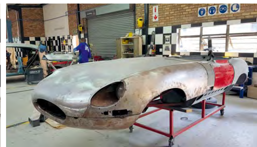
The Jaguar E-Type is starting to look like a car again as we mock up the replacement nose for fitment. It is not a case of simply bolting it onto the hinges and takes a serious number of hours to get just right. We’ve completed the cutting out of rust and replaced what were almost non-existent floors, sills and boot with new metal.
