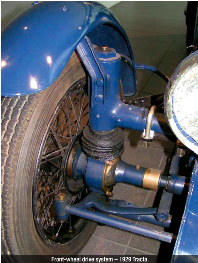
Front-wheel drive system – 1929 Tracta.
