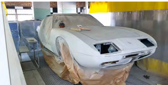
The Maserati Indy is finally in the paint preparation booth. With rust on almost every panel and holes in each crevice it has been a massive job of rotten metal removal, panel making and fitment, and even in primer it’s starting to look like the grand sports car it once was. It will be off to paint next and delivery to the client for assembly is scheduled in the next eight weeks.
