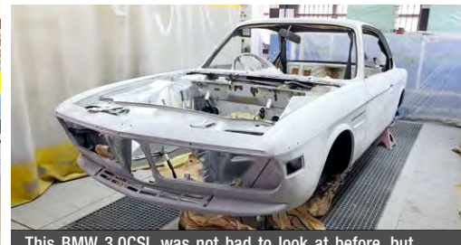
This BMW 3.0CSL was not bad to look at before, but the owner wants it to be the best. With the paint removed, we had to cut out a small amount of rust and rework the fenders to get the correct shape. It's in the preparation booth now and will soon move to the paint shop and be returned to its former glory in original silver. We are overseeing the interior refurbishment and will be assembling soon.
