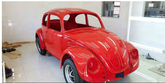
Known as the most powerful production Beetle ever made, the 1600 SP is another one of those South African specials. It's brilliant to see them being added to collections and people spending money to get them right. This one had the usual corroded areas removed and replaced with fresh metal. It is now painted (including the Rostyle wheels) and ready for the owner to collect and put back together.
