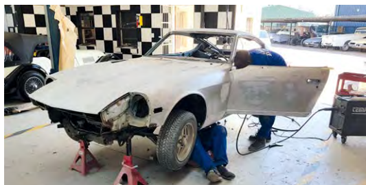
The only Japanese classic in the shop, this Datsun 240Z is making progress again, with the owner having decided on the direction he wants to go. Tin worm took a good hold of the car so new floors have been made and fitted. The areas around the windscreen are next and then we will fine-tune how the doors should hang. It will be painted and shipped off to the owner to put back together.
