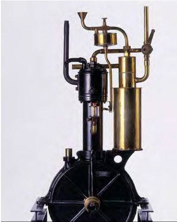
The four-stroke engine developed by Gottlieb Daimler and Wilhelm Maybach, nicknamed 'Grandfather Clock'.
