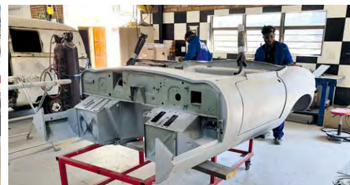
While it looks like not much progress has happened on this Jaguar E-Type since last month, the team has actually been on it full time. There was rust everywhere and this had to be cut out and new metal shaped to replace it. Some new parts were ordered from the UK but it takes many hours of work to get them to fit right. We continue.
