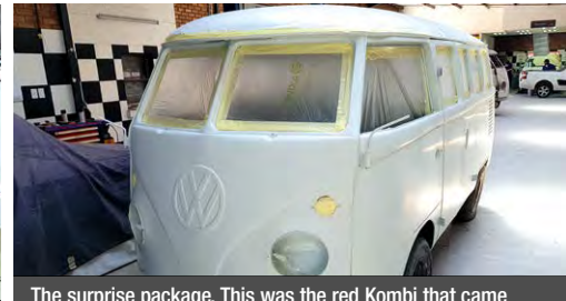
The surprise package. This was the red Kombi that came in looking reasonable. The surprise was that it wasn't. It was packed with filler and fibreglass hiding rust and hail damage. It's been a massive task of cutting and replacing most panels but it finally has a gleaming coat of white paint. Next we will add some green to get the uber-cool two-tone look so desirable on a split-window. The client will assemble.
