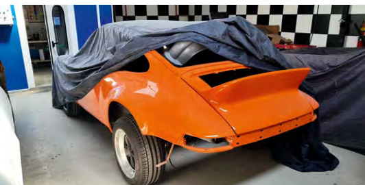
This 1974 Porsche 911 conversion to a '73 RS look was started at another shop but the owner has moved it across to Dino's. The additional fibreglass panels appear to be decent quality but, as with any replacement part, will take some work to fit perfectly. Once this cutting, glassing and shaping is done, we'll paint the entire car in the period-correct orange.
