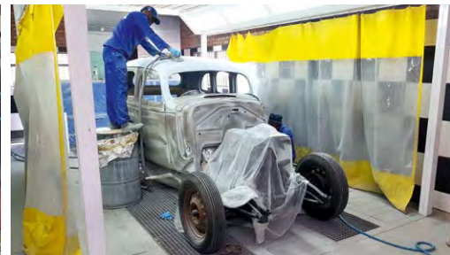
With a rotten wooden frame supporting this Chevy's bodywork, we had to apply some woodworking skills before moving on to the metal. As a result of the poor frame, the panel gaps were insane and needed lots of attention, as did the odd rusty area. We are really proud of the work and it's now ready for paint.
