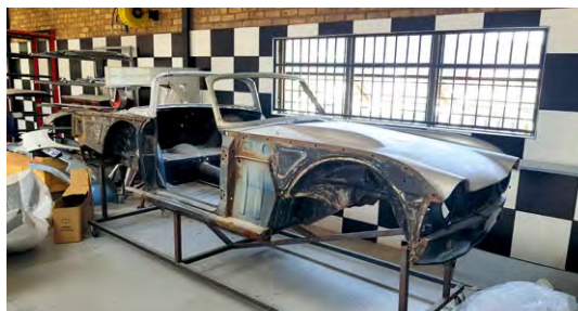
A January arrival, this smart-lined Triumph has come in for a full body repair and paint. It has suffered a bit in the corrosion department and we'll soon get cracking cutting this out before shaping and fitting new metal. We love the Surrey Top - did Triumph beat Porsche's Targa with this style?
