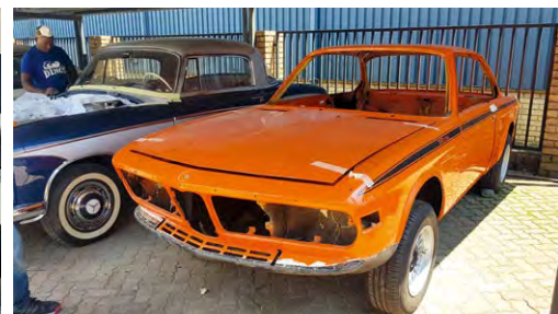
There aren't heaps of BMW's E9 coupés in SA so, with the arrival of this 3.0CSL, we are chuffed to have three currently. This extremely rare lightweight version has thinner metal so it's no surprise we have lots of rust to deal with. Extra careful attention and skill will also be taken while working the aluminium panels.
