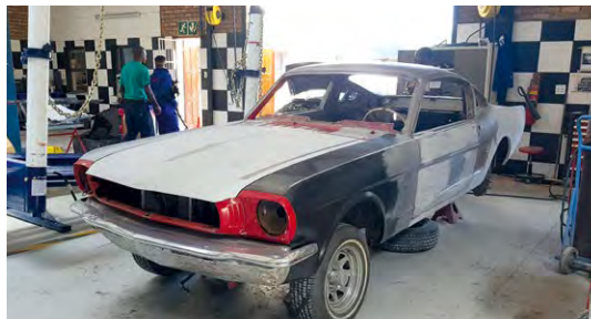
This fastback Mustang was in bad shape on arrival, with rust on almost every panel. We fitted new doors, front wings and bootlid but couldn't find a rear valence. We fabricated a new one from scratch this month and it's now fitted. The once holey 'Stang is getting final adjustments before heading to paint prep.
