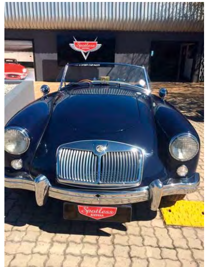
1956 MGA ROASTER. 69 966 miles. 7 years' restoration by previous owner which included an engine rebuild. The car has a telescopic shock absorber system, oil cooler and some extra body fittings e.g. wing mirrors, wind deflectors and wooden steering wheel. R460 000. Phone 082 470 6213.
