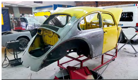
Another Volkswagen Beetle has arrived and, like the many that came through the shop last year, it has suffered at the hands of the dreaded tin worm. While stripping the paint off we are also finding numerous bad repairs, so these along with the rust areas will be rectified with new metal.
