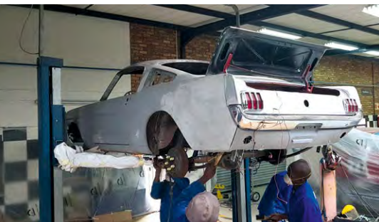
The vast amount of rust that this Mustang arrived with has now been cut out and repaired with new metal. It's up on the lift now so that the undercarriage can be tidied up and any issues repaired before going in for primer and then paint.
