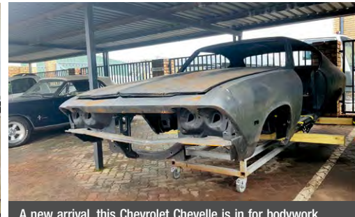
A new arrival, this Chevrolet Chevelle is in for bodywork and paint before the owner assembles the car. Although some new floors have been fitted, there is still a fair amount of rust that needs to be cut out and repaired. The bonnet is too far gone so this will be the only new panel sourced.
