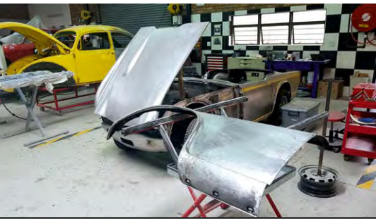
Progress on the Triumph is moving along well. As far as old British cars go it was reasonably sound, but we have had to remove sections of rust and make up some new panels. It's not too far from the primer stage and we await instruction on what colour to paint it.
