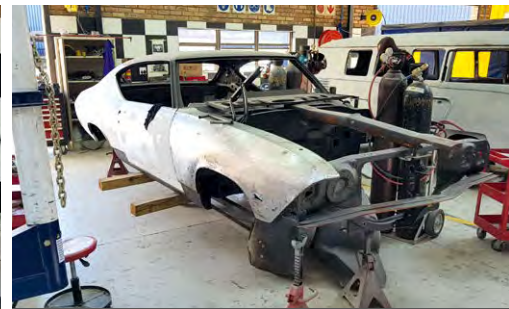
A new addition to the workshop, this Chevrolet Chevelle has had some panels replaced by a previous shop, but we've taken over. There's still heaps of rotten metal, which we are removing and making new. Except for the bonnet, this is too far gone so will be imported.
