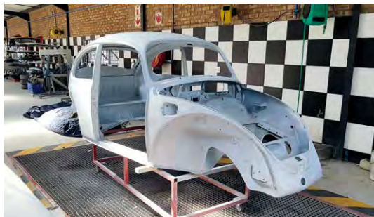
Another air-cooled VW to go through the process. This one needed the usual removal of rust and making of new metal panels. It has now been primed and is waiting at the doors of the spray booth. It will be assembled by Generation Old School.
