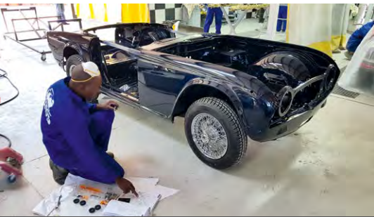
After having some rust removed and body imperfections corrected, the Triumph TR has received its final coat. The client delivered a restored chassis and we are fitting the wing beadings and chassis to body rubbers as per the book. He'll then take it home to finish.
