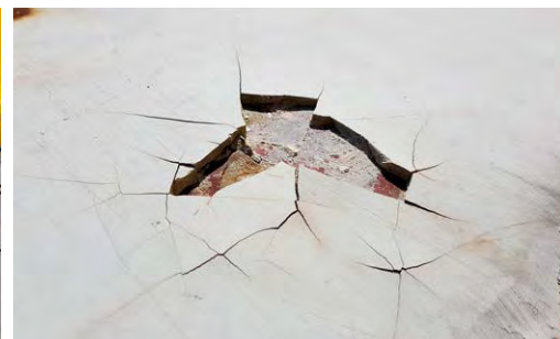
When this Kombi came in it didn't look too bad, but when we removed filler that was around 10mm thick from the roof, it revealed a structure that looked more like a doily than metal. We sourced a second-hand roof, repaired this and then grafted it onto the VW Kombi. This meant lots of bracing and careful cutting in order not to damage or warp the topless shell. The surgery has gone well and it's now getting more minor issues fixed.
