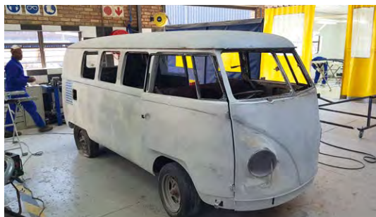
When this Kombi came in it didn't look too bad, but when we removed filler that was around 10mm thick from the roof, it revealed a structure that looked more like a doily than metal. We sourced a second-hand roof, repaired this and then grafted it onto the VW Kombi. This meant lots of bracing and careful cutting in order not to damage or warp the topless shell. The surgery has gone well and it's now getting more minor issues fixed.
