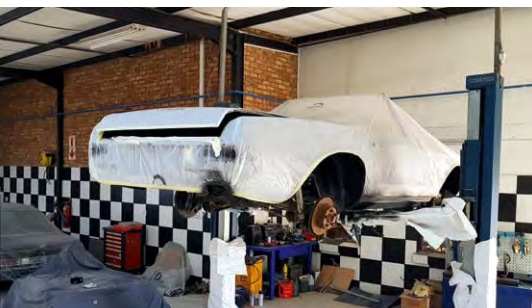
One of the biggest jobs of the year, this Mercedes SL had plenty of damage hidden by filler. The top half is complete and now we are redoing the floors, which were covered in sound-deadening material to hide the rot. We've made new floors from scratch.
