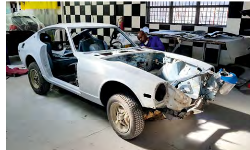
The Datsun 260Z has been sitting for a month or so while we waited for some imported replacement parts. The headlight surrounds were the final delivery. Rust and gremlins have been removed and we are fitting the final touches before priming and painting.
