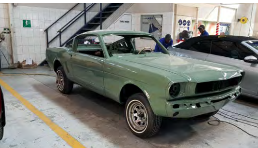
It's moments like this that make it all worth the effort. This Mustang took hours of labour, with almost every panel having the rot cut out and replaced with newly shaped metal. The customer chose the most beautiful shade of green. It's ready for them to assemble.
