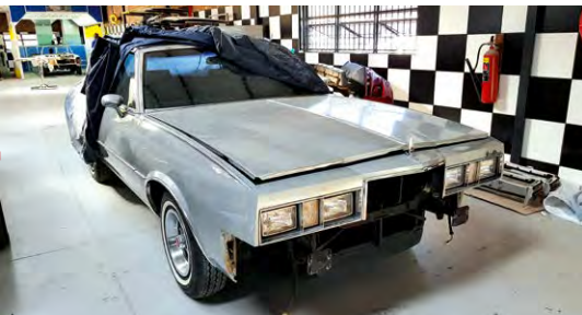
This, a Pontiac Grand Prix, is one awesome bit of 1980s America and is in for some plastic surgery. The rubber/plastic bumpers have not aged as well as the rest of the car and have cracked extensively. We are repairing and filling these before painting to match the existing bodywork.
