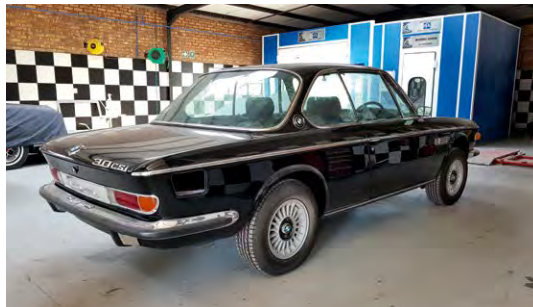
The end is in sight for our own BMW 3.0CSi. It's all new, with body and paintwork redone, reupholstered seats, dash and carpet refurbishment and any damaged exterior trim or lights replaced. We've imported engine bay stickers and now await the engine.
