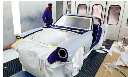
It's been a relatively long job on the Datsun 260Z with numerous parts needing to be imported. Rust has been cut out, metal replaced and fit sorted out. And now it gets its final paint before the customer takes it to assemble.
