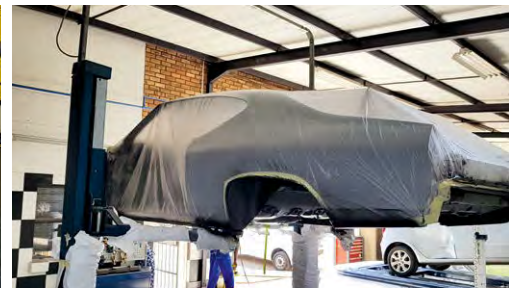
This Chevrolet Chevelle has had some panels replaced by a previous shop, but there was heaps of rotten metal which we removed and replaced. Only the bonnet was imported; the rest of the replacement parts were made locally. It's now ready for the paint booth.
