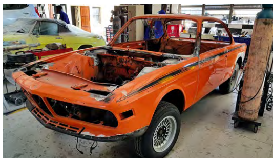
This rare BMW 3.0CSL has lived a hard life – if the panel damage is anything to go by. A UK import, it also has a lot of the dreaded tin worm. We are cutting this out and replacing with newly made sections. Thankfully the aluminium doors, bonnet and boot aren't too bad.
