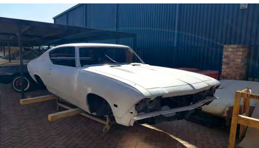
Another monstrous Chevrolet Chevelle in the shop, and another monstrous pile of rotten metal was left on the floor. We've cut this all out, fabricated new bits and fitted some replacement panels. It's now being prepped for primer and then paint.
