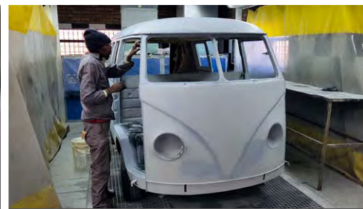
This VW splittie Kombi should perhaps have been left on the rubbish dump but following many long hours it's now as good as new and being prepped for paint. To get it to this stage, we had to source a better roof section and graft it onto the original shell, remove plenty of rotten metal and fill countless holes.
