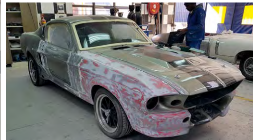
This is the second replica Eleanor Mustang to visit Dino's. Like the first, it was a recent build that looked nice from far but far from nice. The owner has booked it in for a full-body job. We are in the process of taking off the paint, fixing any blemishes and repairing the fibreglass additions.
