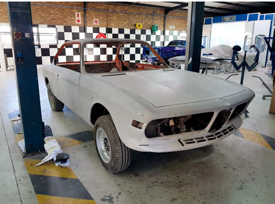
We are extremely happy with how this rare BMW 3.0CSL is turning out. It had lived a hard life and had clearly seen some salt roads. It's been a massive task cutting out the tin worm and making up replacement sections. Careful dent work on the fragile aluminium doors, bonnet and bootlid has paid off and thankfully these don't need to be replaced.
