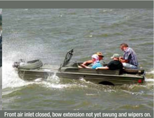
Front air inlet closed, bow extension not yet swung and wipers on.
