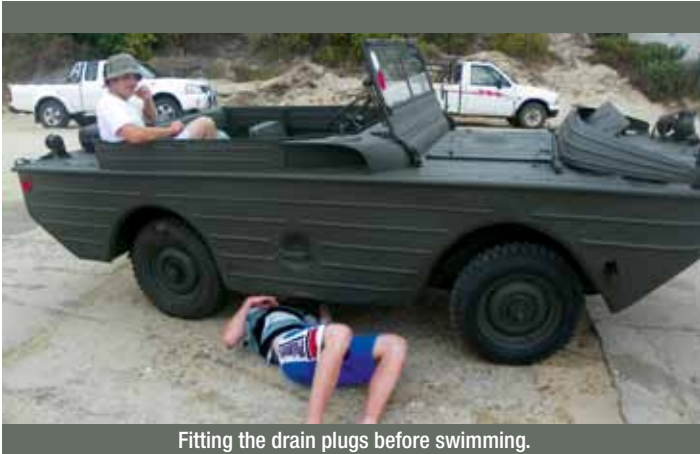
Fitting the drain plugs before swimming.
